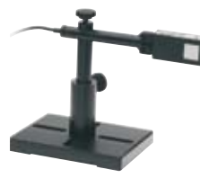
PD300 with filter installed
